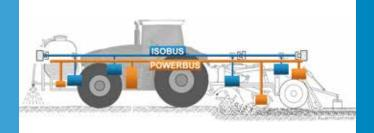
Electric drives are becoming increasingly important in agricultural technology. The only thing that has long been missing is a standardized interface for direct and/or alternating current that is able to channel enough power from the tractor to the implement to drive large electric motors.
