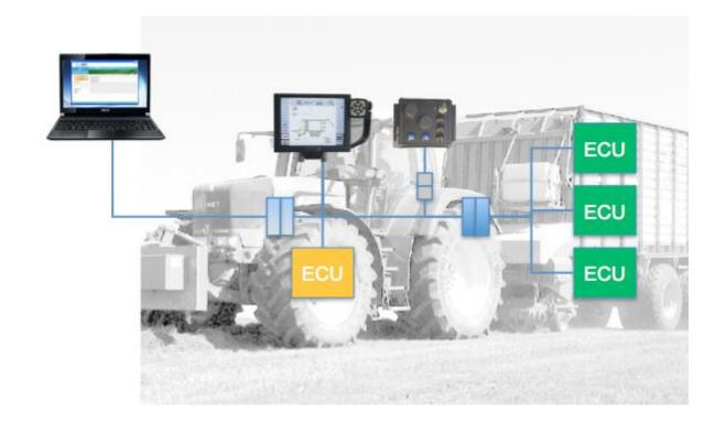
The service technician arrives, connects a laptop to the Universal Terminal (UT) in order to read out the diagnostic data with the AEF ISOBUS Check. The AEF ISOBUS Check application generates a diagnostic file.
