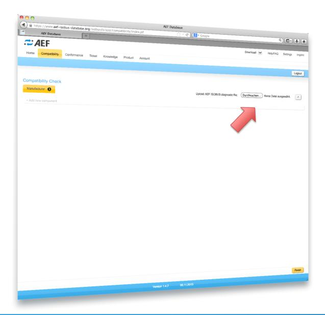
Then the service technician accesses the AEF ISOBUS Database, logs in to his account and uploads the diagnostic file directly into the system via an upload function.
