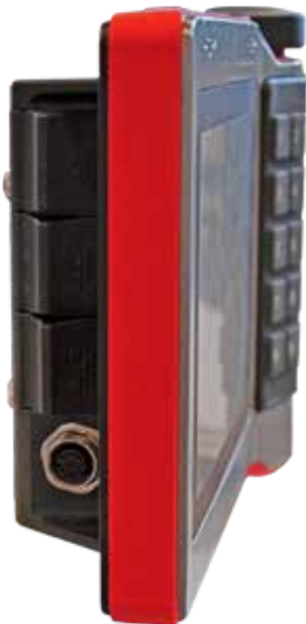
ISOBUS terminal with camera plug contact
